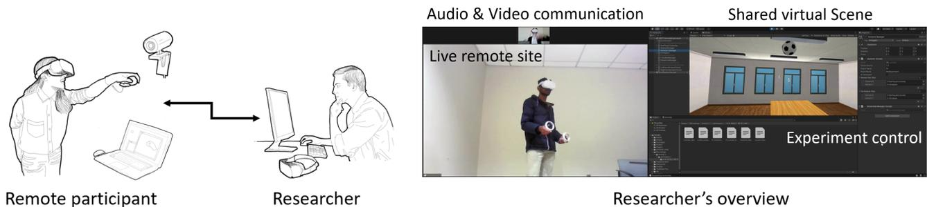
**Figure 1:** *RemoteLab* is a novel open-source Unity toolkit that enables synchronized play of a user study over multiple sites. The researcher can view the VR scene shared among participants, control the experimental conditions, and intervene if needed, such as guiding a participant through filling a questionnaire in VR (left).
